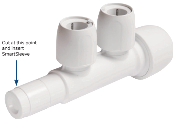
Figure 62: Cutting a Key manifold spigot end
