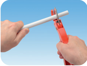
Figure 14: Hep 2 O Key jointing sequence
