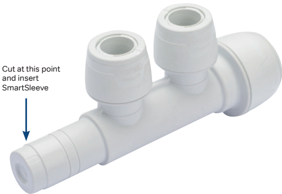
Figure 64: Cutting a Keyless manifold spigot end
