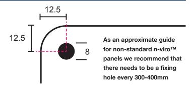
For n-viro™ graphic panels that require non-standard fixing holes - bespoke requirements must be discussed prior to placing orders.
