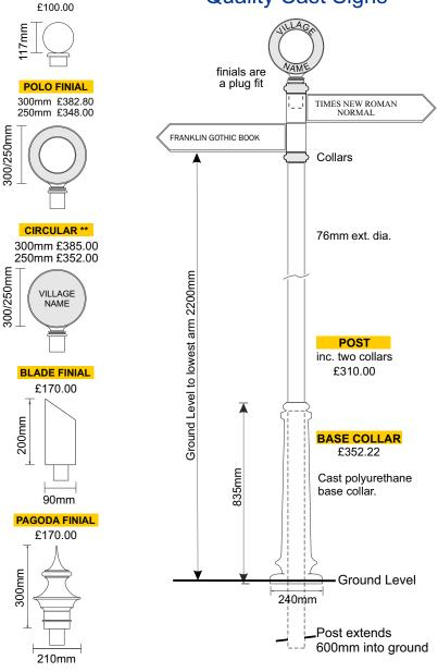
Fingerpost arms & circular or bespoke finials are cast in aluminium. Base collars, ball & pagoda finials are cast in polyurethane.
