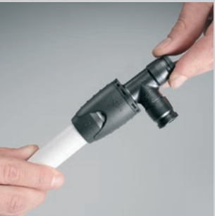
Push until the pipe is completely inserted and visible through the spyhole
