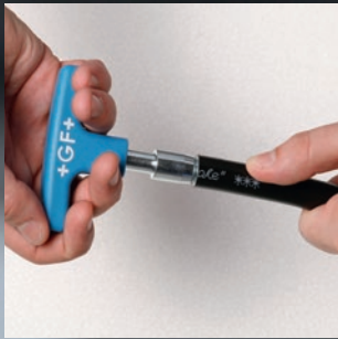
Calibrate the pipe
