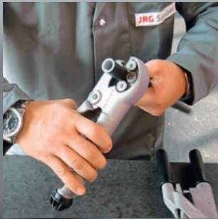
Cut the pipe
